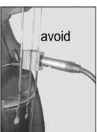
Never pull the cable or handle the sensor by the cable
