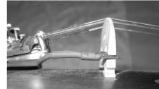
It will be necessary to watch quite particularly the parallelism of surfaces in contact. The pickup has to, during placement, force enough. Beware to not break the auricle during that operation. If the sensor is too loose and does not force enough, it can be tighten up with a thin piece of wood (or cardboard) on it top
